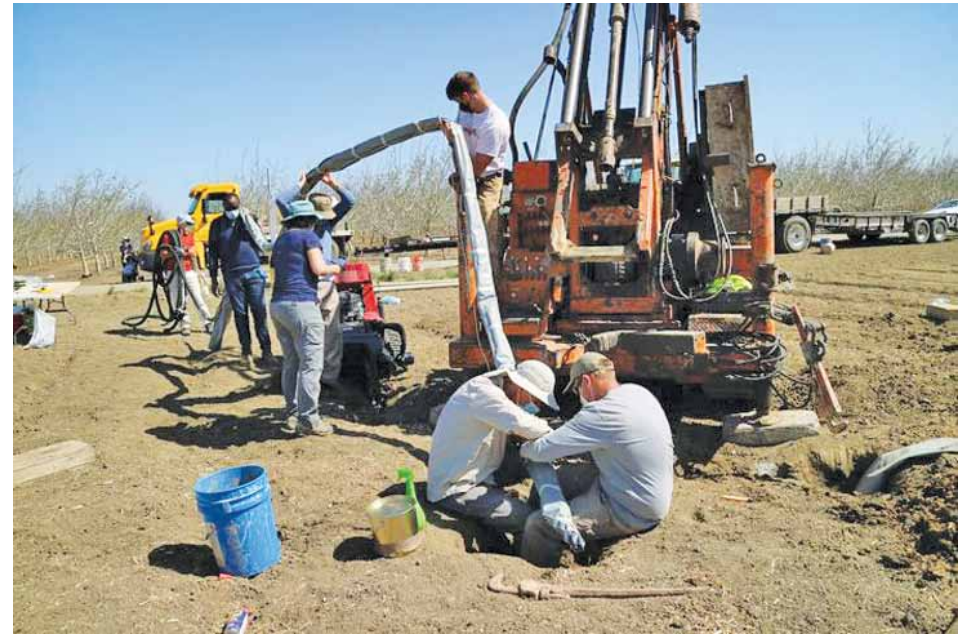
Measuring contaminants at UC Davis: UC Davis researchers insert a device that continuously collects water samples underground, providing real-time data on nitrate contaminant movement. (Isaya Kisekka, courtesy of UC Davis)
