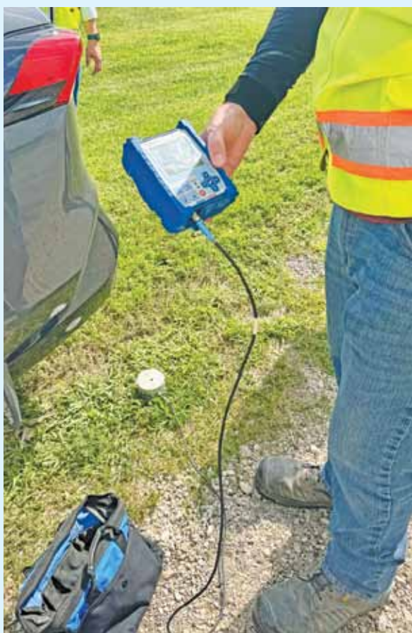
Mike keeps a close watch on his PPV meter, the small screen acting like a traffic light for the entire operation. If the ground shakes too much, he's the one who calls it off.
