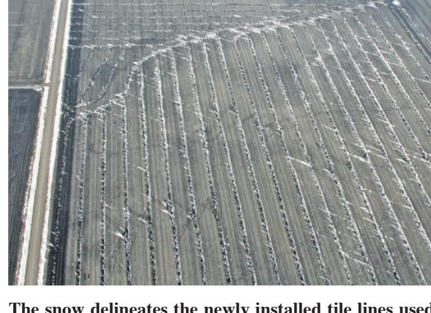
The snow delineates the newly installed tile lines used to drain excess water from the farm field.
